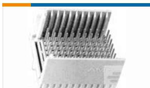
TE 系列/零件编号5646457-1 2MM HM,ASY,T-F,PIN,088 POS
